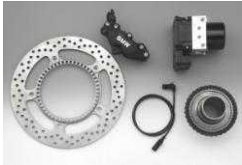
Figure 33: BMW, elements of an ASC systems
