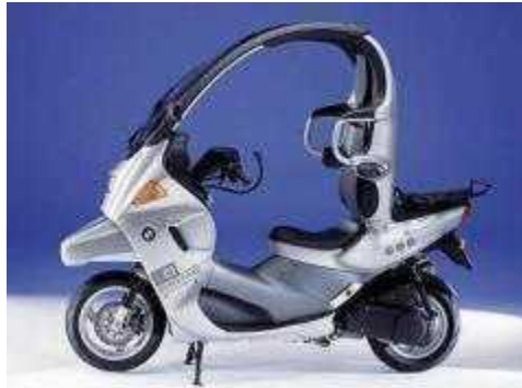
Figure 36: BMW C1 scooter with protective cage 32
