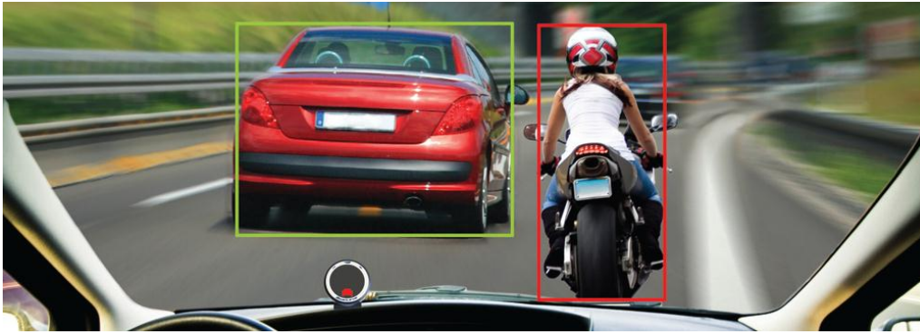
Figure 40: PTW detection by FCW system 36
